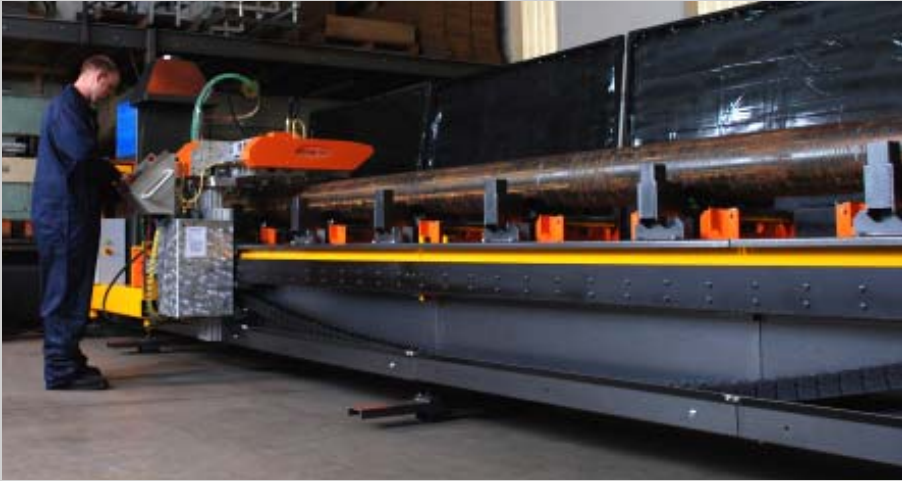
W-244 Computer-Controlled Pipe cutter with Four-Axis Control for controlled bevels and deep weld penetration
